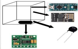
**We will put the device on a person's hand and the** Arduino Nano will take up data from MAX 30100 sensor and the **Thermistor**. The device needs to be attached to the body by using a wrist strap i.e. a Velcro. Then the thermistor needs to be placed below our arm and the MAX 30100 sensor will be placed under the device as because the device will have some weight and that pressure will be applied on the sensor thus the sensor will receive the data more precisely.
