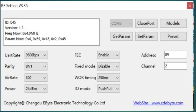
RF\_Setting\_EN.exe is the windows software to set the module.
